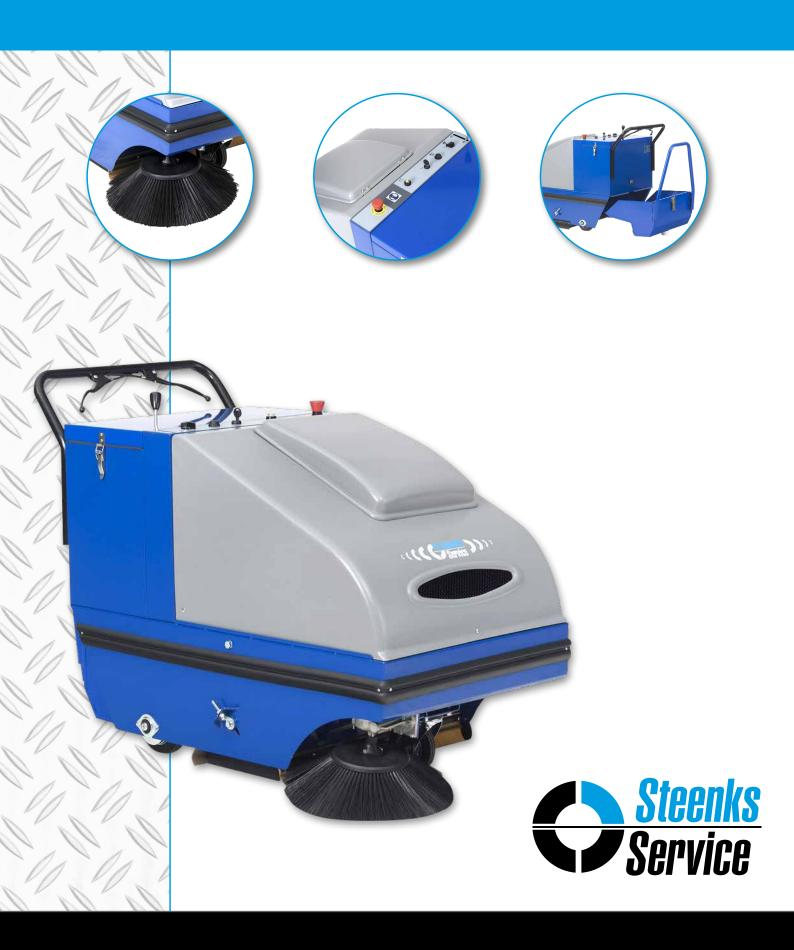
The Stefix 75 is a robust floor sweeper with a sweeping width of 750 mm. The 5 m<sup>2</sup> dust filter makes this machine extremely suitable for sweeping bulky waste as well as fine dust particles. The front wheel electric drive and simple controls mean that a cleaning capacity can be achieved of 3,400 m<sup>2</sup> surface area per hour.
