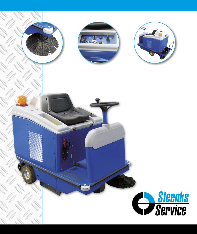
The Stefix 95 is a robust floor sweeper with a sweeping width of 925 mm which can be extended using an extra side brush to 1,150 mm. The 6 m<sup>2</sup> dust filter makes this machine extremely suitable for sweeping bulky waste as well as fine dust particles. The front wheel electric drive and simple controls mean that a cleaning capacity can be achieved of 6,200 m<sup>2</sup> surface area per hour.
