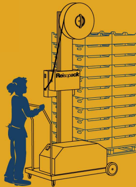
This simple system assists edge protector placement on the first strap.
