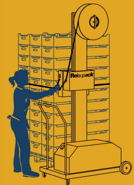
This simple system assists edge protector placement on the first strap.
